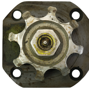
SPROCKET WEAR WITH OFF-BRAND GATHERING CHAINS
