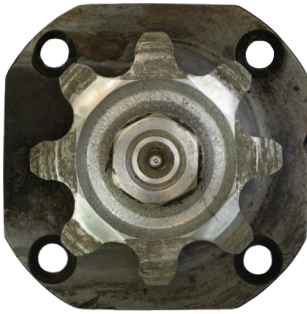
SPROCKET WEAR WITH DRAGO GATHERING CHAINS
